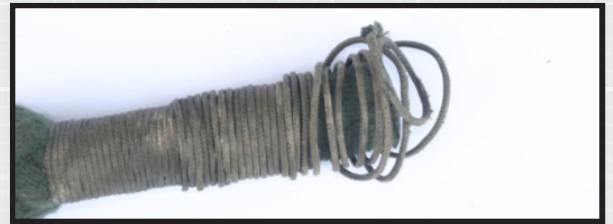
Picture 3: End whipping damaged and must be replaced
